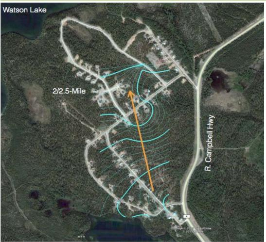
Figure 6. Piezometric contours for 2/2.5-Mile area. The orange arrow indicates the global flow direction.
