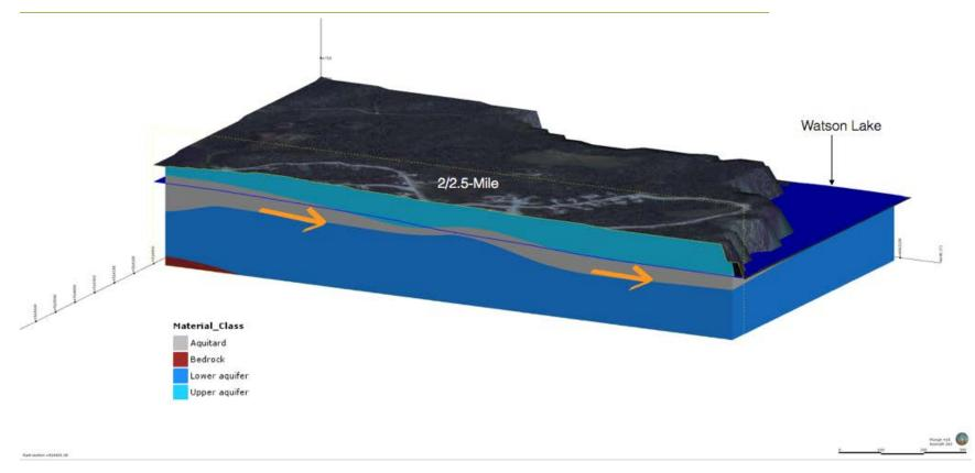
Figure 4. Interpolated water table for 2/2.5-Mile area. Section scene of the model taken along a South-North axis, looking South-West. The orange arrows indicate the groundwater flow direction.
