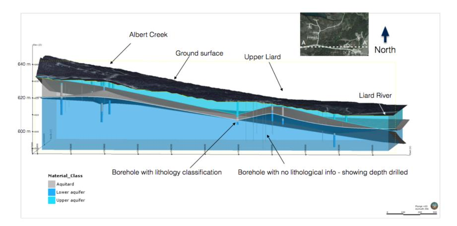
Figure 1. Hydrogeological interpretation of borehole lithologies in Albert Creek and Upper Liard. Section scene of the model taken along the Alaska Highway, looking North.
