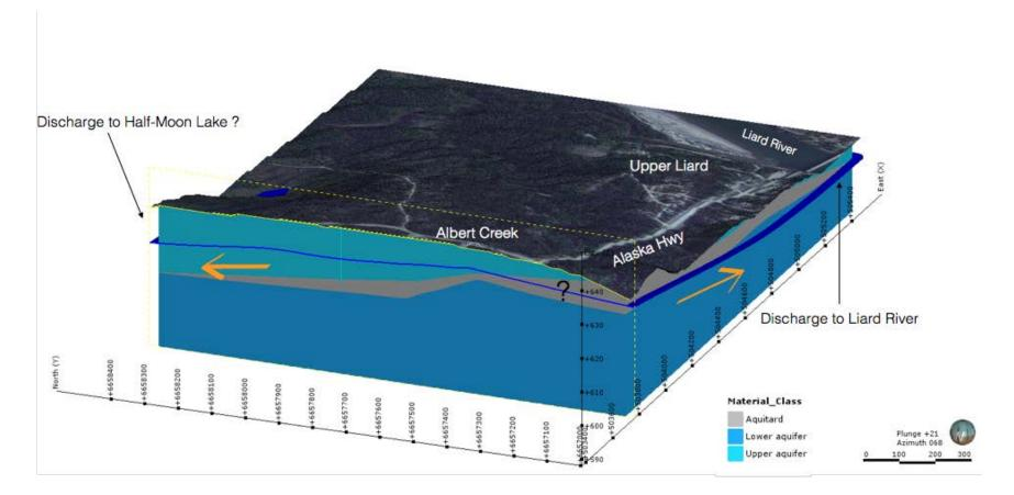
Figure 3b. Interpolated water table for Albert Creek and Upper Liard area. Section scene of the model taken along the Alaska Highway, looking North-East. The orange arrows indicate the groundwater flow directions.
