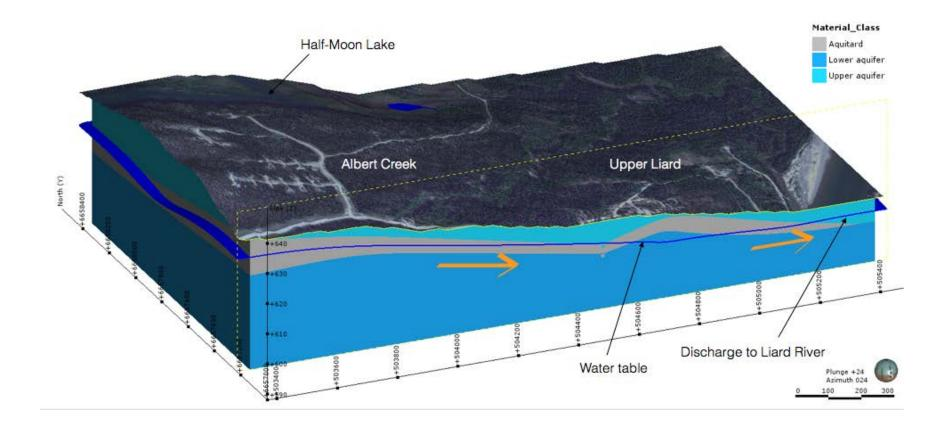
Figure 3a. Interpolated water table for Albert Creek and Upper Liard area. Section scene of the model taken along the Alaska Highway, looking North-East. The orange arrows indicate the groundwater flow direction.
