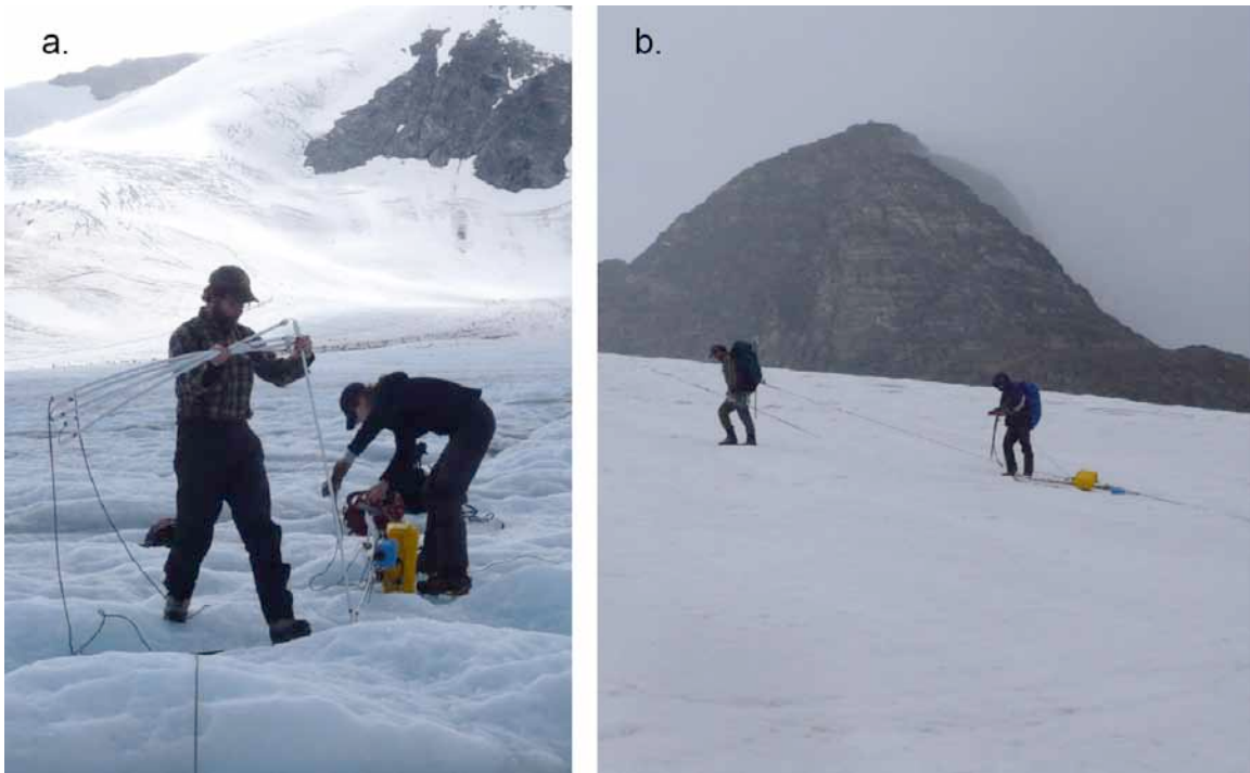
Figure 5. The system and its associated hardware components were mounted on skis with flexible plastic tubing protecting the antennae, and the entire system was pulled on foot and guided over the glacier surface by the field research team. The photos show the setup and deployment of the radar system on glaciers within Fantail Basin: a) connecting plastic tubing to stabilize and secure antennae for travel over the complex ice surface; b) towing the radar unit over the glacier surface.
