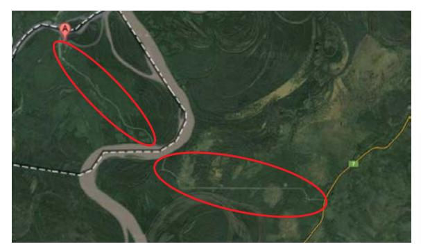
**Figure 14b.** A new 23 km, all-weather access road was opened to Nahanni Butte in 2010 and runs from Highway #7 to the east bank of the Liard River. A water taxi crosses the Liard River in the summer, and an ice road is used in winter, and then the access road continues to the community of Nahanni Butte.
