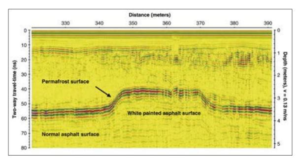
Figure 8. Radargram of Ground Penetrating Radar (GPR) (Jørgensen and Andreasen, 2007).
