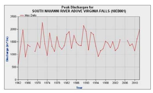
*Figure 17.* Maximum daily discharges observed over a 51-year period from 1962 to 2012 at the 'South Nahanni River above Virginia Falls' gauge station.
