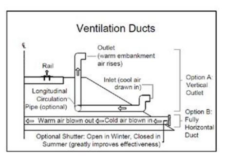
Figure 10. Ventilation duct design (Regehr et al., 2012).
