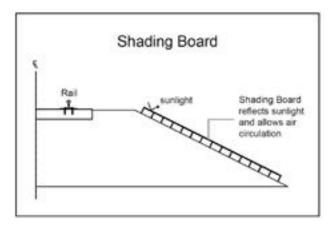
*Figure 7.* Conceptual diagram of shading board (Regehr et al., 2012).
