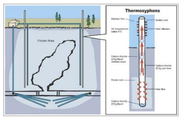
*Figure 6.* The frozen block method uses thermosyphons to ensure subsurface contaminants remain frozen through time. This system is being used for the Giant Mine remediation project near Yellowknife, NWT (INAC, 2007).
