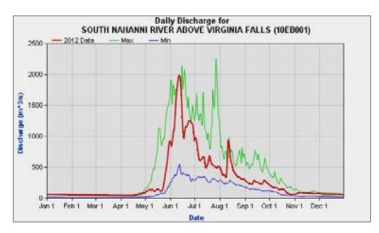
*Figure 16.* Statistical comparison of the 2012 daily averaged discharges to maximum daily discharges observed over a 71-year period from 1942 to 2012 at the 'South Nahanni River above Virginia Falls' gauge station.
