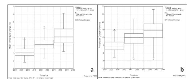
**Figure 5.** Boxplots of MAT (**5a**) and MAP (**5b**) projections from an ensemble of ~140 GCM projections for Atlin-Taku Plan Area and surrounding region. Middle line and box represent median; top and bottom of boxes represent 75th and 25th percentiles, respectively. Whiskers are 1.5 times interquartile range (IQR), + symbols indicate minimum or maximum outside IQR. Source: PCIC Regional Analysis Tool, http://pacificclimate.org/tools/regionalanalysis.
