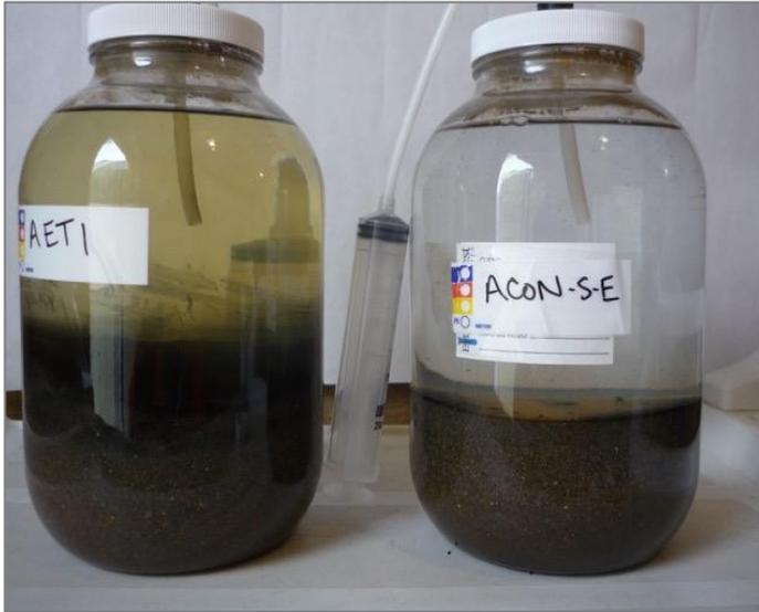
**Figure 9.** Comparison of ethanol bioreactor (containing inoculum and ethanol)(left) and control bioreactor (containing ethanol, but no inoculum)(right) at T=150. The ethanol bioreactor had a substantial black precipitate, whereas the control had very little (a clear effluent).
