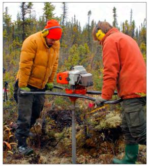
**Figure A1.** Photograph of the GÖLZ<sup>™</sup> portable Earth-drill system used for permafrost coring.
