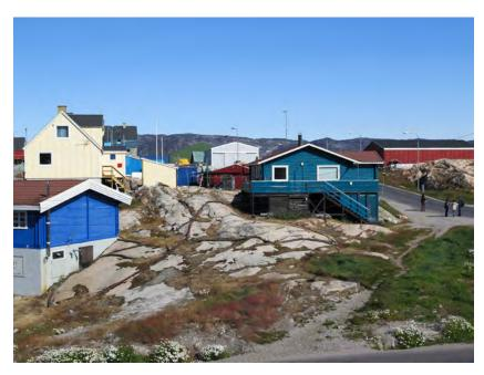
*Figure F1.* Houses in Ilulissat, western Greenland, built directly on bedrock.
