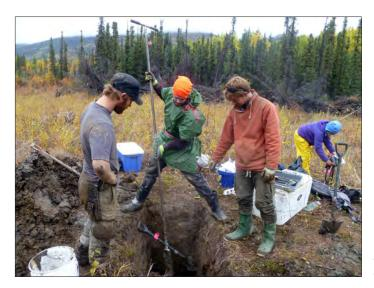
*Figure A5. Photograph of the hand auger, used for permafrost coring.*
