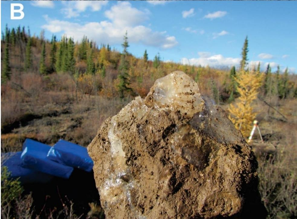
**Figure 2.4 Permafrost observed during culvert installation at site km 381. A- ice-rich fine grained soil excavated below the embankment; B- close-up of an ice-rich permafrost sample collected during the excavation works**
