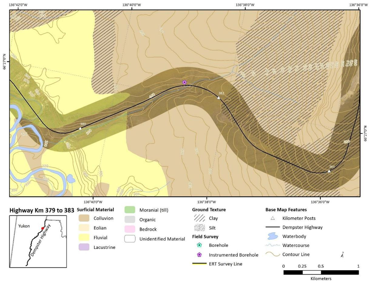
Figure 2.2 Surficial geology map for the Culvert Site at km 381
