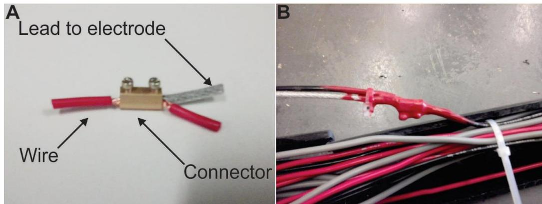
**Figure 3.6 ERT wire/electrode wire assembly. A- Connection; B- liquid plastic coating.**
