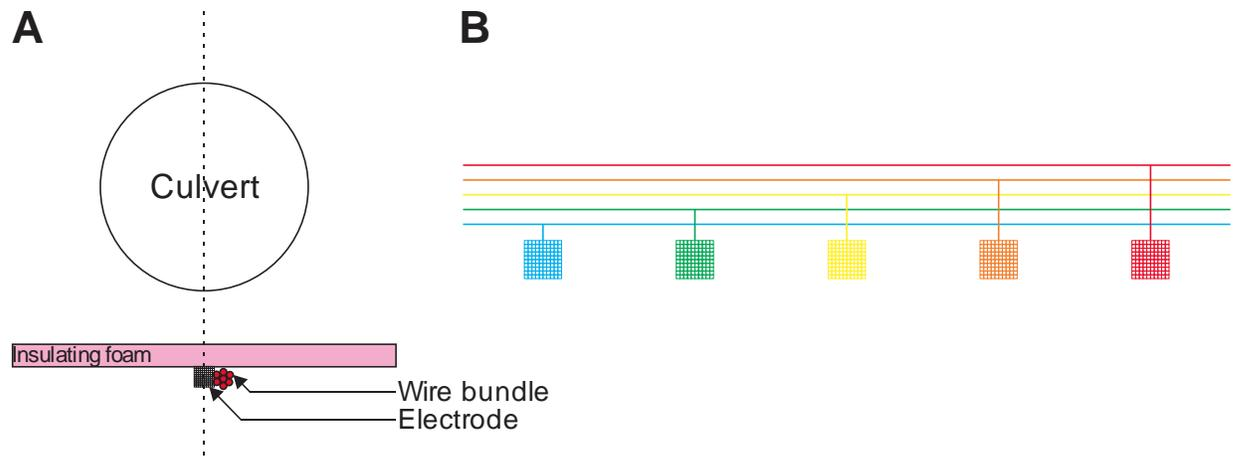
**Figure 3.5 electrodes and wires arrangements; A- Location of the electrodes relative to the culvert axis and insulating foam; B- Connection of each electrode of individual wire on a regular spacing.**
