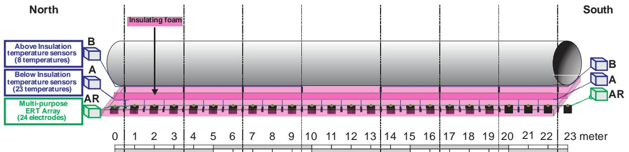
**Figure 3.1 Instrument setup of the culvert at km 3xx of the Dempster Highway**
