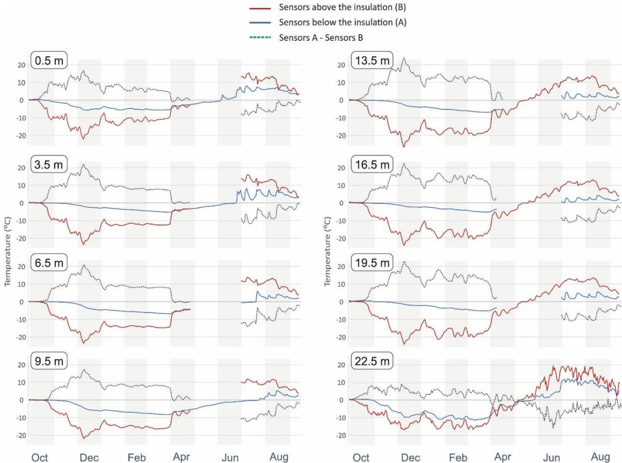
**Figure 4.3 Comparison between temperature recorded below and above the foam, at similar locations.**
