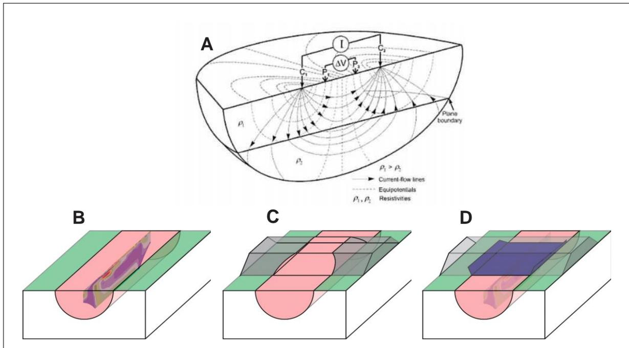
**Figure 3.4 Principle of the use of ERT survey under an embankment, with insulating foam providing a barrier to electricity. A: diagram of electrical propagation in the ground; B- standard ERT survey; C- ERT survey under embankment without insulation; and D- ERT survey under embankment with insulation**
