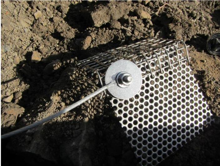
**Figure 3.7** Stainless-steel mesh and perforated plate electrode.
