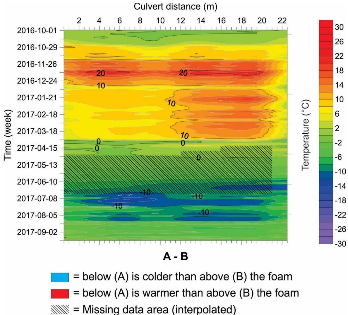
**Figure 4.5 Evolution of the difference of temperatures between array A (below the foam) and array B (above the foam) recorded along the culvert during one year. Blueish tones mean that temperature below the foam are colder, below and above the foam. Reddish tones mean that temperature below the foam are warmer.**
