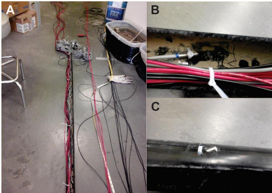
**Figure 3.8 ERT and temperature wires bundles. A- ERT and temperature are attached together.; B- internal view of the protective ABS piping; C- external view of the protective ABS piping, allowing contact between sensor and soil.**
