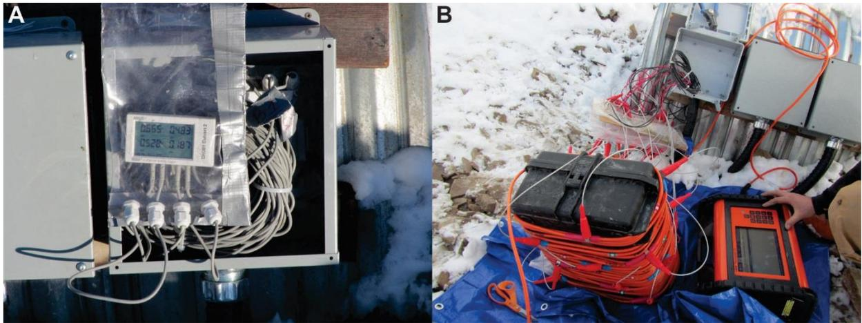
**Figure 3.13 Instrumentation such as installed on the main culvert. A- 4-channel Hobo temperature logger in steel case; B- ERT wires connected for a test run on NCE's ABEM ERT system.**
