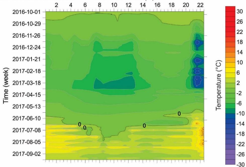
**Figure 4.4 Evolution of the temperatures recorded all along the culvert during one year, below and above the foam.**
