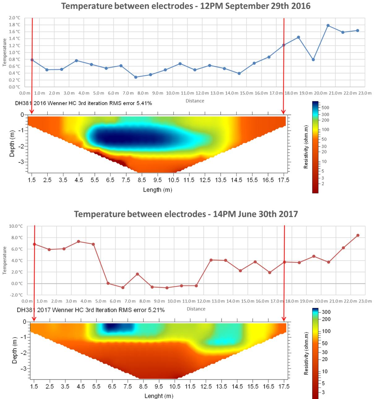
**Figure 4.7 Comparison between ERT survey performed in September 2016 and June 2017 and temperature recorded below the foam at the same time.**
