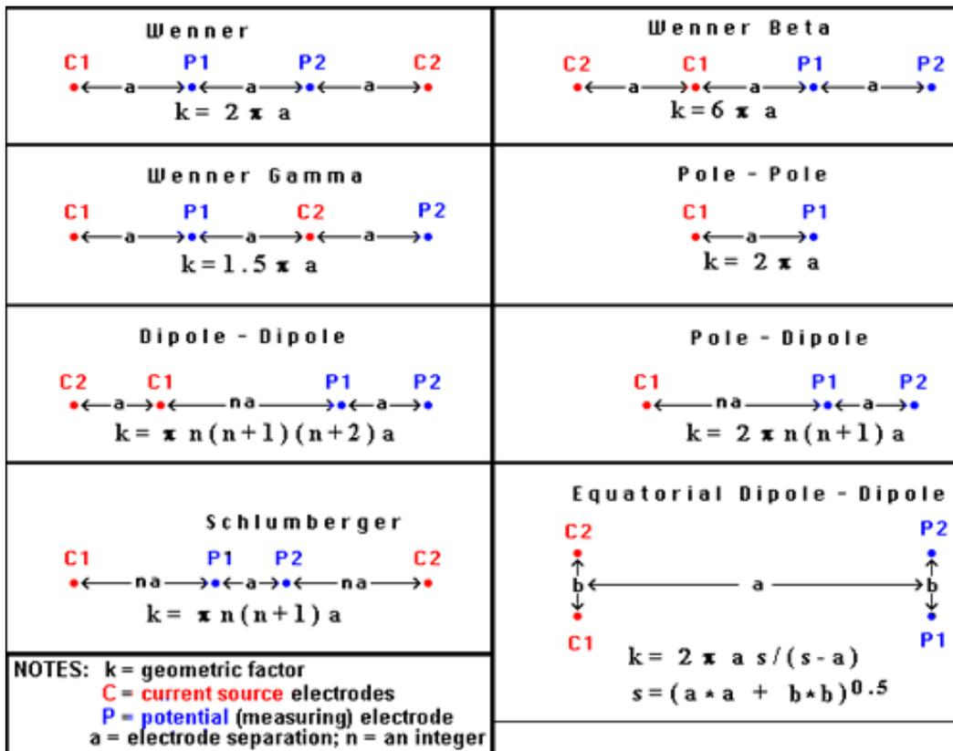
**Figure 3.3** Survey configurations or “arrays” for ERT surveying.
