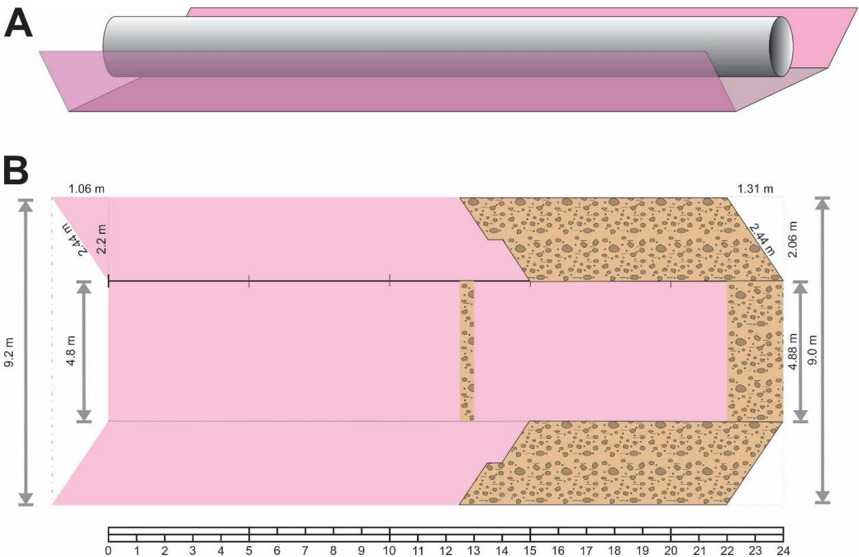
Figure 3.12 Diagram showing foam installation compared to initial design. A- Original U-shape design (3D view); B- final installation with missing insulated areas (brown, gravelly pattern).
