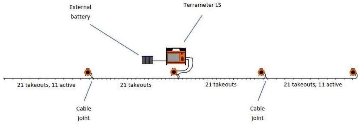
**Figure 3.2 Instrument set-up for ERT surveying**
