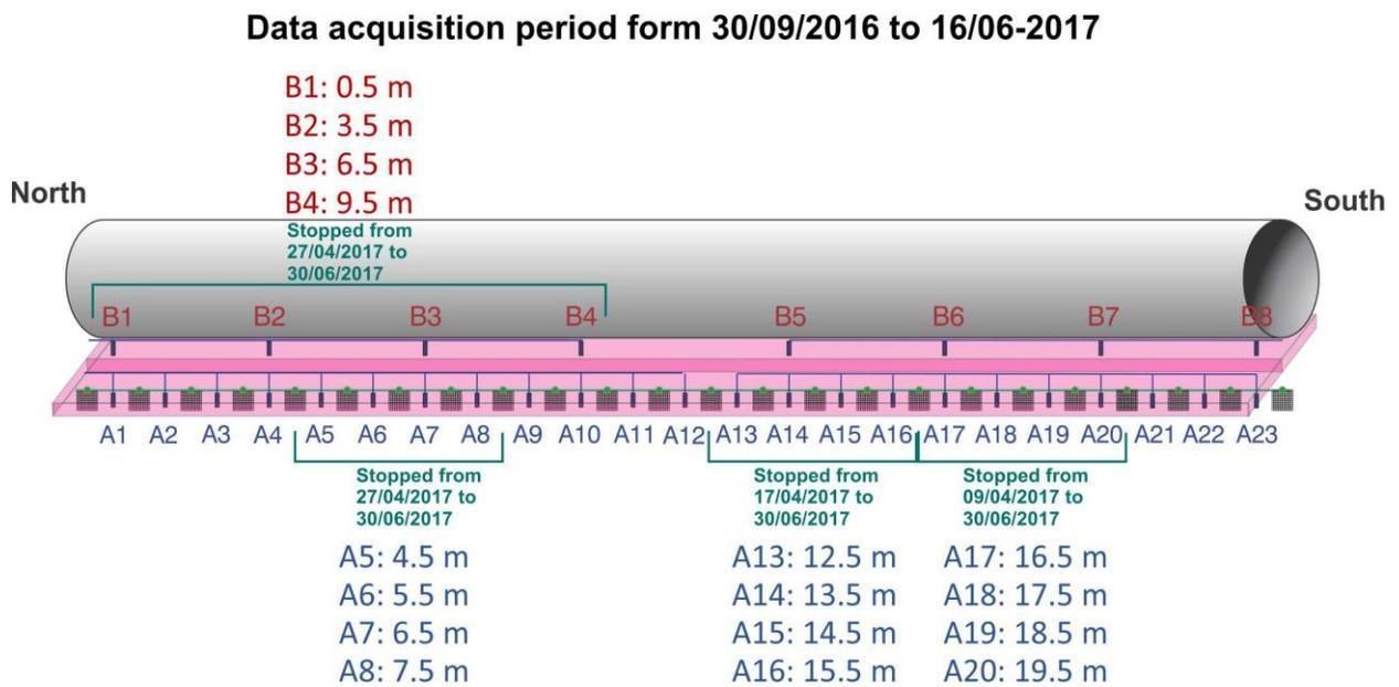
**Figure 4.2 Diagram showing what were the loggers and sensors affected by premature shutdown.**
