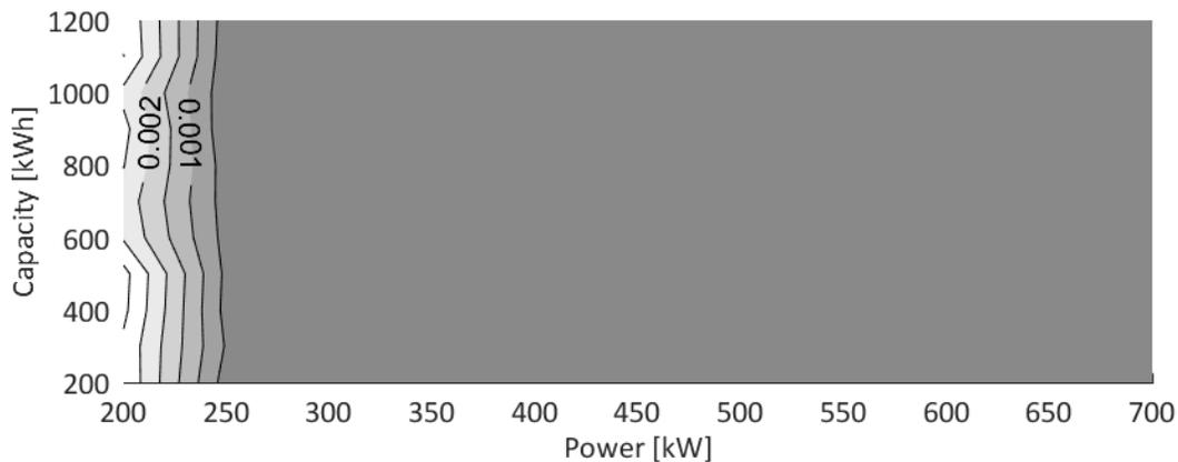
**Figure 9: Levelized cost of insufficient power resulting in a blackout.**
