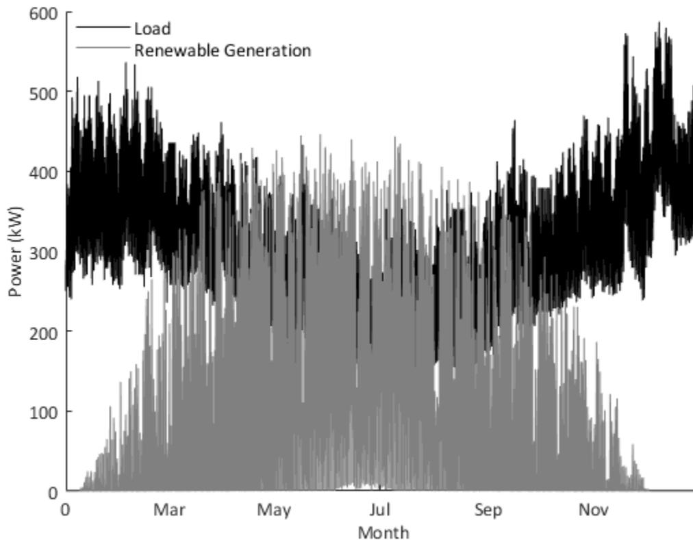
**Figure 3: Energy demand of Old Crow and the predicted solar generation profile over one year.**
