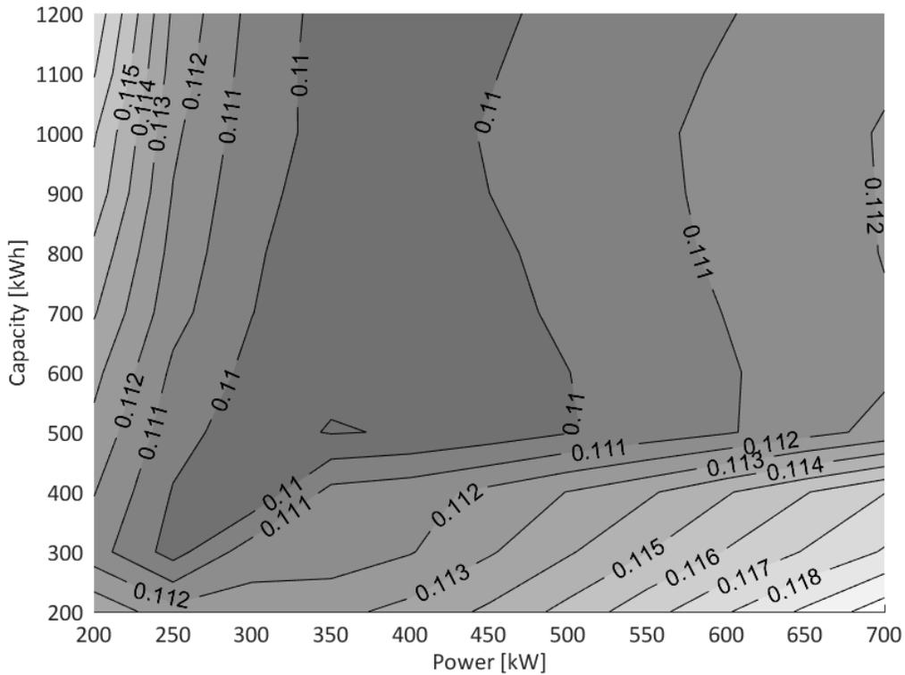
**Figure 13: Total leveled cost of energy with weighting factors focusing on avoiding insufficient power and blackout events.**
