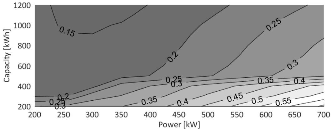
**Figure 5: Levelized cost of energy for the capital cost of power rating.**
