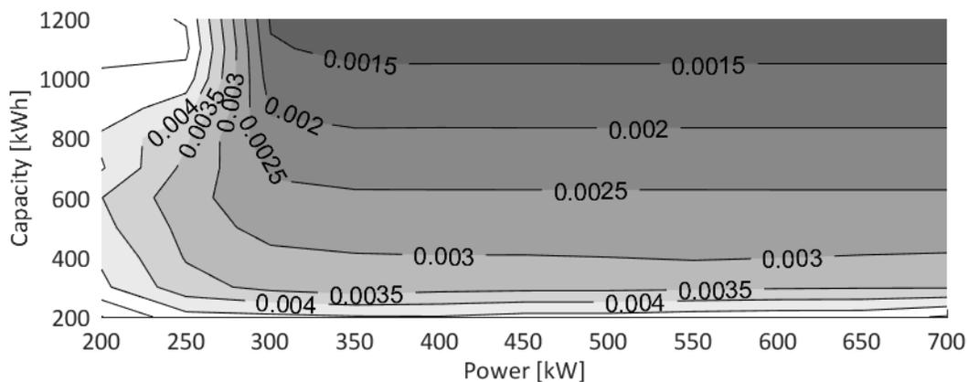
**Figure 7: Levelized cost of curtailed energy.**
