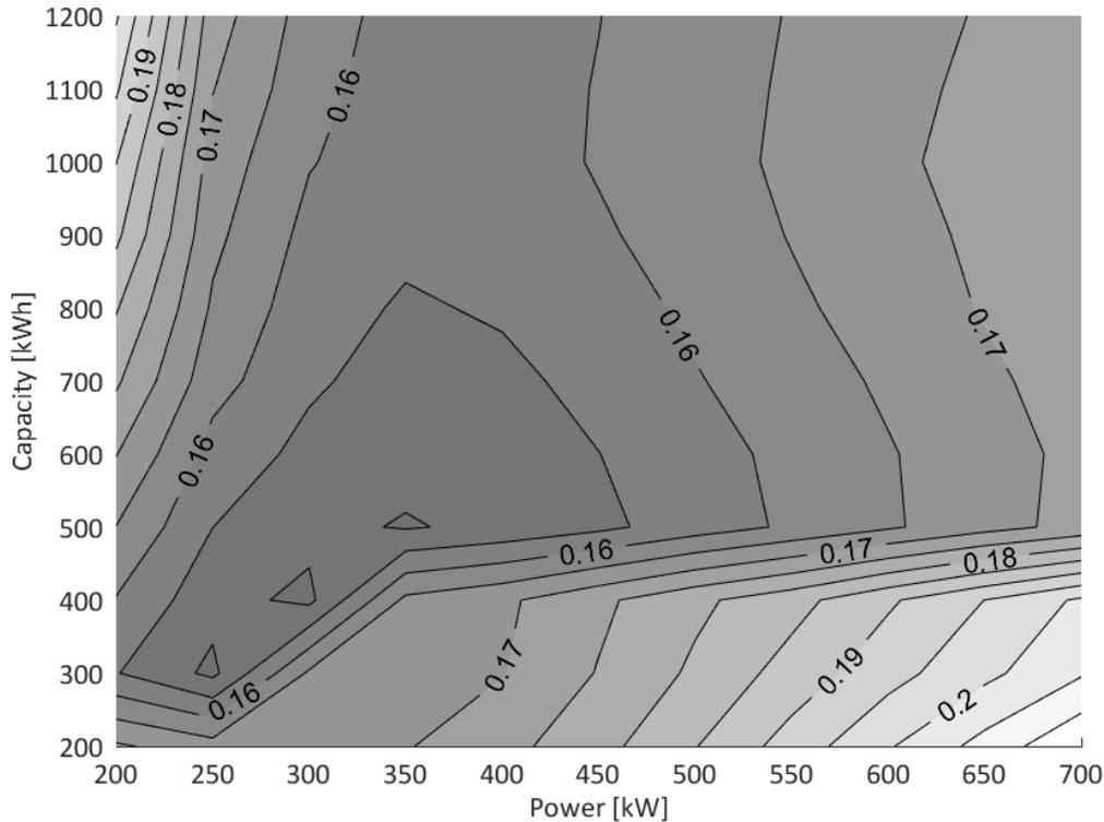
**Figure 11: Total levelized cost of energy for all parameters with equal weighing factors.**
