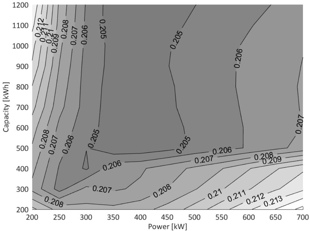
**Figure 12: Total levelized cost of energy, weighting factors focused on fuel consumption and curtailment**
