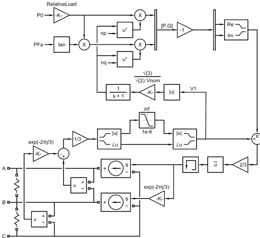
**Figure 2: Dynamic load model used to represent loads on the isolated grid**
