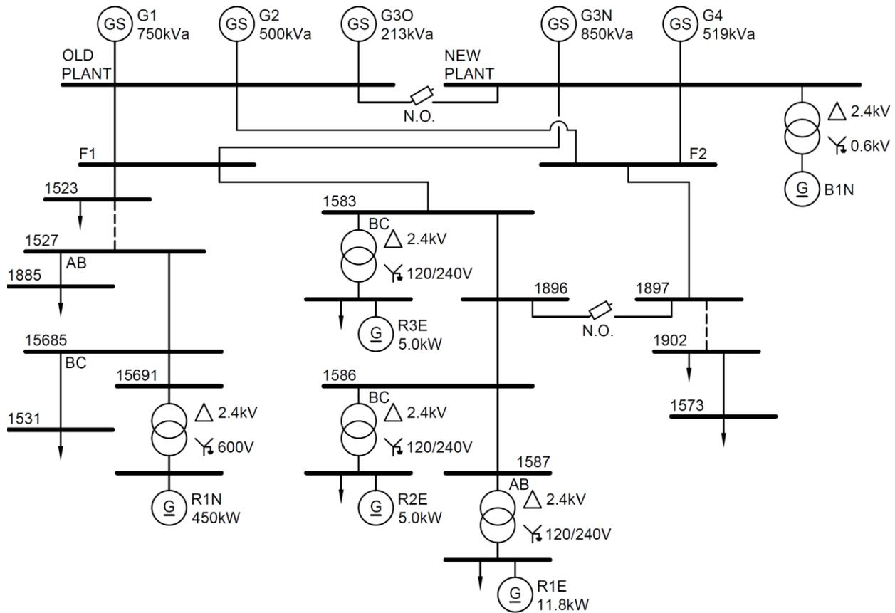
**Figure 1: Single line diagram of Old Crow Yukon isolated electrical grid**
