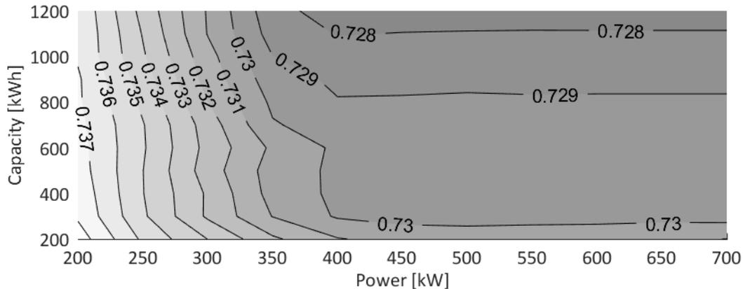
**Figure 6: Levelized cost of the fuel consumption of the generator plant.**
