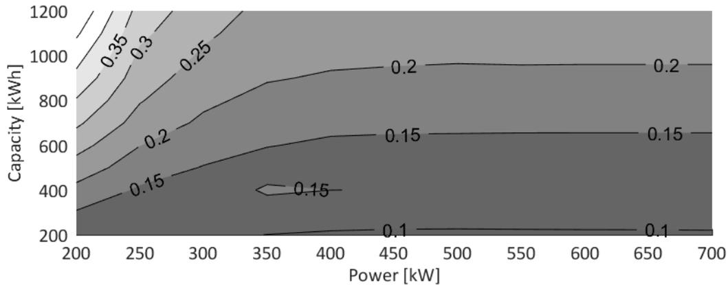
**Figure 4: Levelized cost of energy for the capital cost of energy capacity.**
