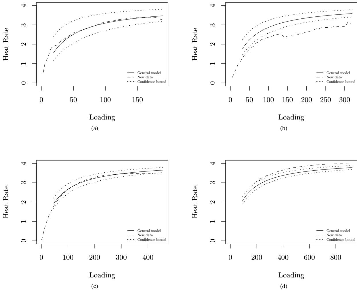
Fig. 6: Comparisons of new genset data to general fuel consumption model results. (a) compares a 190 kW genset, (b) compares a 320 kW genset, (c) compares a 457 kW genset, and (d) compares a 925 kW genset. The model has very close approximations for (a) and (c), and less close but still reasonable approximations for (b) and (d).
