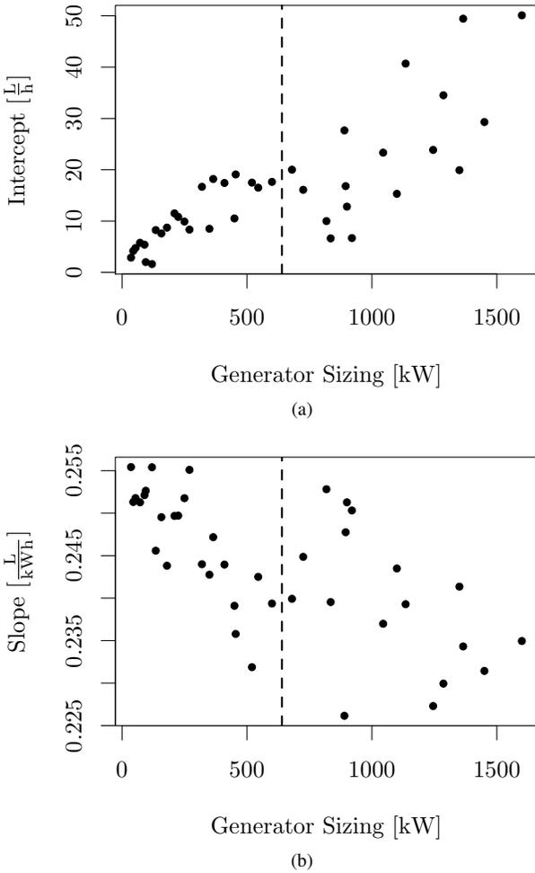
Fig. 4: Multilevel regression estimates of fuel consumption (a) intercept and (b) slope across generator sizing. The dotted vertical lines emphasize an apparent “break” in the data.
