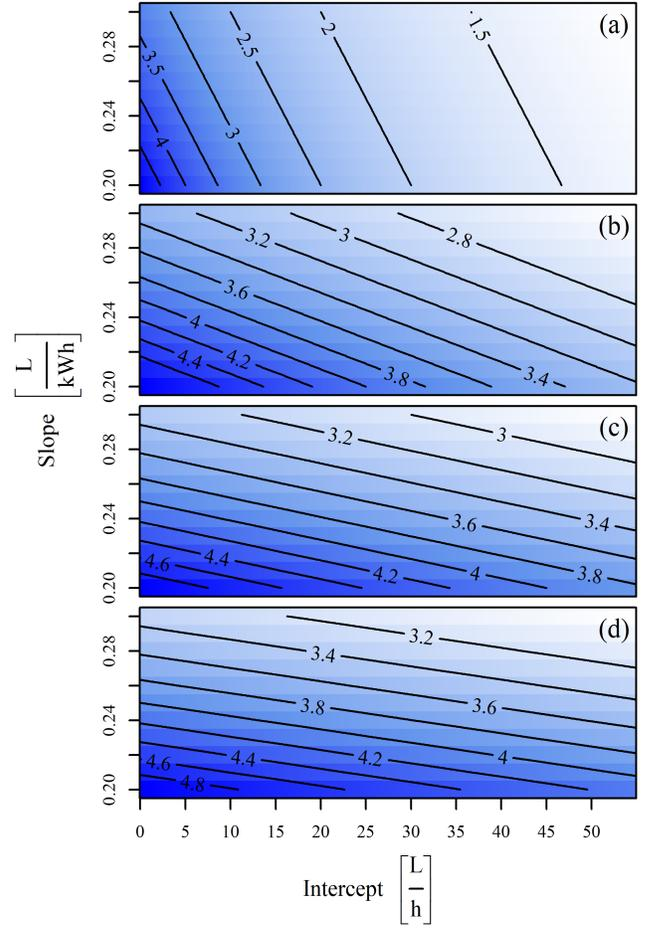
Fig. 3: Contours of the heat rate curve in (2) as a function of estimated slope and intercept range at a (a) 100 kW loading, (b) 500 kW loading, (c) 900 kW loading, and (d) 1300 kW loading.
